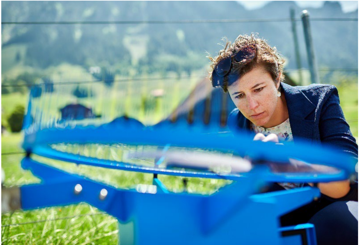
Installation of hail sensors
